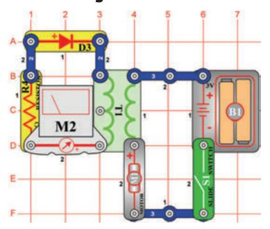
OBJECTIVE: To measure the current through a transformer.
