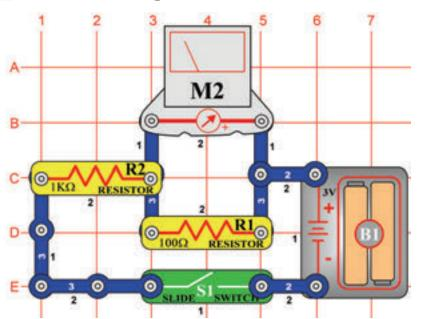
Set the meter (M2) to the LOW (or 10mA) scale. Inside the meter, there is a fixed magnet and a moveable coil around it. As current flows through the coil, it creates a magnetic field. The interaction of the two magnetic fields cause the coil (connected to the pointer) to move (deflect). By itself, the meter can measure 300µA. To increase its range, resistors are connected in parallel or in series to the meter.
