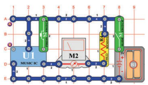
Set the meter (M2) to the LOW (or 10mA) setting. Instead of driving a speaker (SP) with the music IC (U1), you can see it by using the meter. Turn on the slide switch (S1) and the meter deflects according to the rhythm of music. After the music stops, hold down the press switch (S2) to make it continue.
