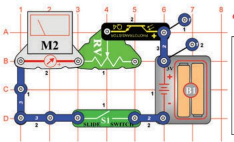
Set the adjustable resistor (RV) to the far left and turn on the slide switch (S1). The circuit is now very sensitive to light. Wave your hand over the phototransistor (Q4) and the meter deflects to the left, almost to zero. Move the adjustable resistor to the far right and see how less sensitive the circuit is to light now.
