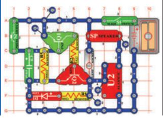
Replace the 1-snap wire from the middle snap on U2 with a 2-snap and connect it to grid location D7 & E7. The circuit now produces a different sound. Change R5 and C5 with the following combinations for R5 and C5:
