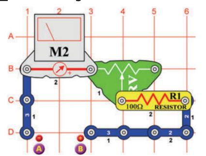
Build this 0-3V voltmeter circuit. Set the meter (M2) to the LOW (or 10mA) setting. Using new batteries, place the battery holder between points A & B. Adjust the adjustable resistor (RV) so the meter deflects
