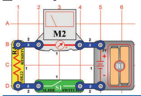
Set the meter (M2) to the LOW (or 10mA) setting. The meter indicates the amount of current in the circuit. Turn on the switch (S1), the needle deflects indicating the amount of current. The  $10k\Omega$  resistor limits the current, otherwise the meter could be damaged.
