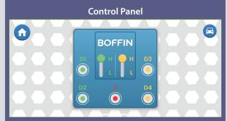
CP has 5 outputs (D1, D2, D3, D4 an A) which are controlled by the app. Outputs D1-D2 and D3-D4 are paired so that each hcontrols a motor in both directions and they can be used to set one of the two levels output voltages, called H (high) and L (low). Output A has a low power output that can control the horn (W1), but cannot control the car's wheel motors. Use the app to control them.
