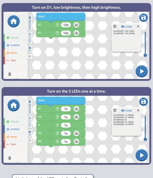
Limitations of the U33 controller: Controller has only circuit outputs (no inputs), so it cannot make measurements or decisions based on anything happening in your circuit. Also, the A output on the controller can only supply low currents, so it cannot be used to control the car motors directly.
