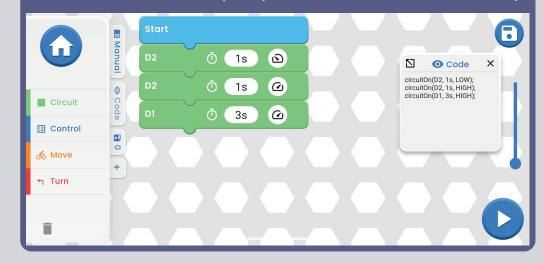
**Part B, Beep & Flash:** Replace motor (M1) with the speaker (SP2), then create the program shown here.
