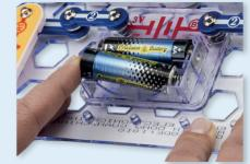
When installing a battery, be sure the spring is compressed straight back, and not bent up, down, or to one side. Battery installation should be supervised by an adult.
